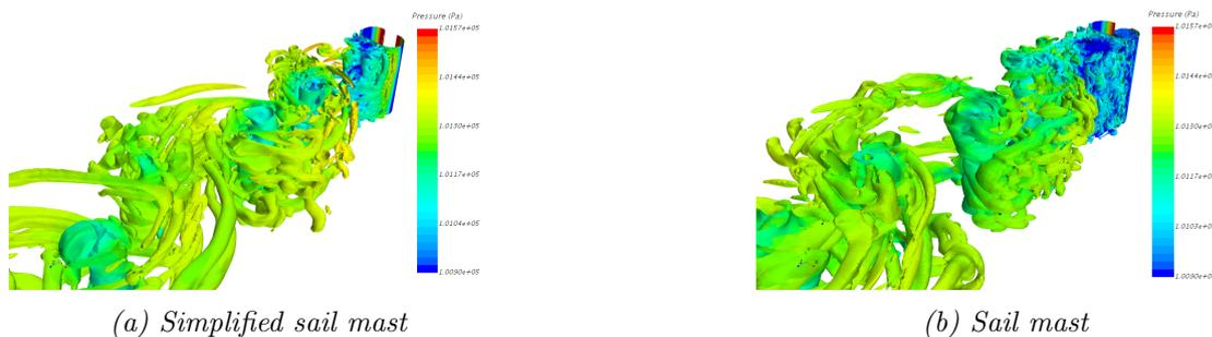
Figure 5.15: Flow structures colored by pressure at  $\psi = 90^\circ$
