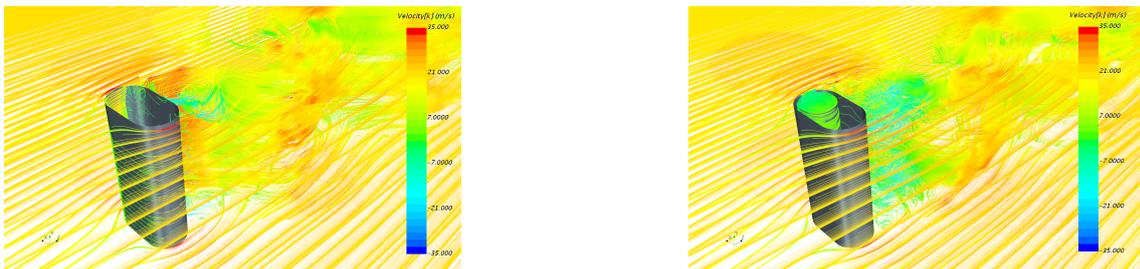
Figure A.2: Streamline colored by velocity in stream wise direction at  $\psi = 90^\circ$
