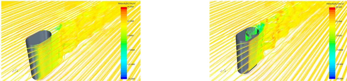
Figure A.1: Streamline colored by velocity in streamwise direction at  $\psi = 0^\circ$
